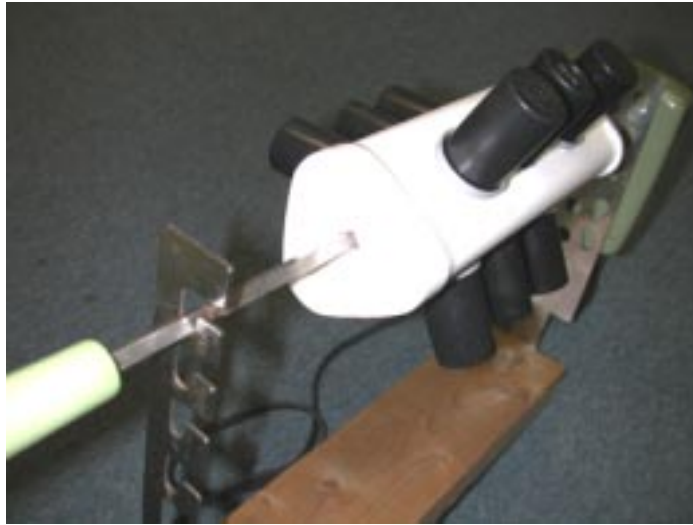
Figure 4. A clinostat made from a rotisserie.
